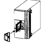
e. To remove, push the Eject button next to the slot and pull slide out from the scanner.
